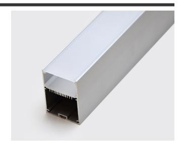
For modern architectural commercial lighting designs, our aluminum profile "P7" is a perfect solution. Aluminum channel "P7" can accommodate up to two rows of high-output LED strips, with an inner dimension of 1.60" (40.6mm) wide, and properly disperse heat generated by the strips. The housing features an integrated "slot" to hold an LED driver or power-supply effectively allowing users to create their own light fixtures for general lighting applications.
