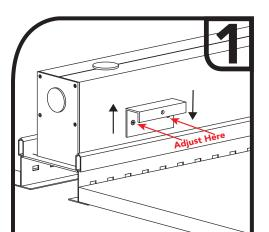
Adjust grid bracket as needed to accomodate your grid structure using the screws shown.
