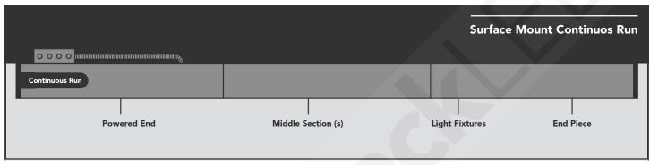
\*Fixtures do not include conduit, they have "knock-outs" to receive conduit
