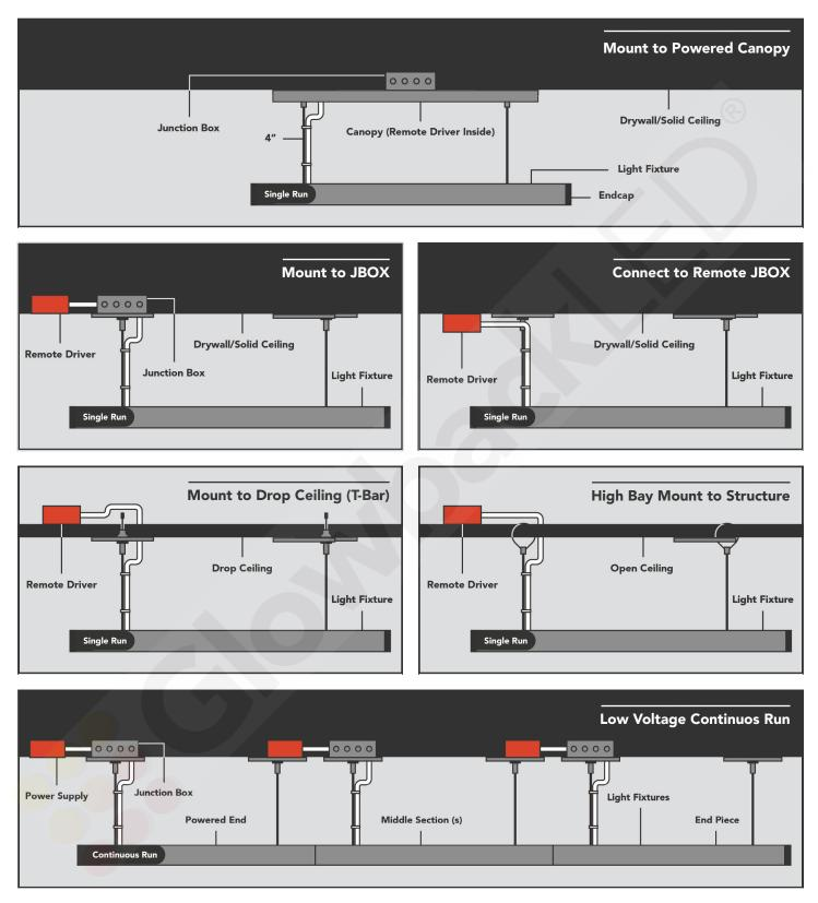
\*Remote Power Supplies MUST be left accessible, they cannot be installed behind finished ceilings.
