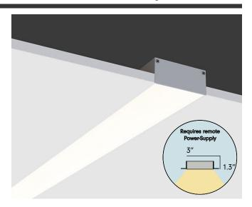
Our LVLBY3T is a 3 inch wide recessed trim-less ("plaster-in") architectural linear recessed light available in tailor-made custom lengths. It is available in 350 or 900 lumens per foot light output levels and can be used to illuminate residences, retail spaces, and high end offices. Our LVLBY3T features an integrated plaster-bead that allows one to sand and finish ("mud up") right to the diffuser leaving a clean 3 inch wide line of lighting with no visible trim or flange.
