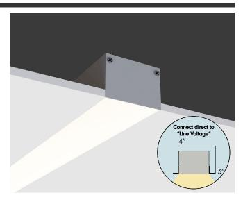
Our LVLBY43T is a 4 inch wide recessed trim-less ("mud-in") architectural linear recessed light fixture. It features an integrated plaster bead which allows one to sand and finish ("mud up") right to the diffuser leaving a clean 4 inch wide line of lighting with **no** visible trim or flange. Our LVLBY43T features an integrated power supply allowing one to connect the fixture directly to the "line voltage" source of the home or building (120-277 or 347VAC Input).
