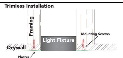
**Framing Required!** Build framing on either side of light fixture.
