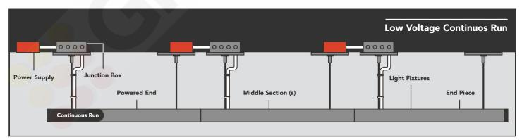
\*Remote Power Supplies MUST be left accessible, they cannot be installed behind finished ceilings.
