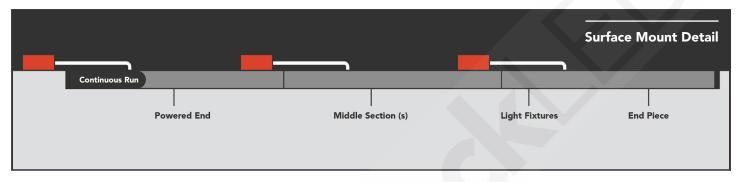
\*Remote Power Supplies MUST be left accessible, they cannot be installed behind finished ceilings.
