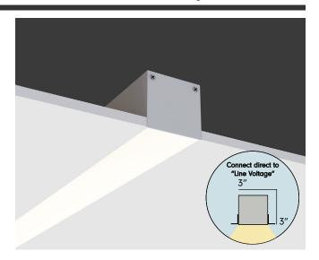
Our LVLBY33T is a 3 inch wide recessed trim-less ("plaster-in") architectural linear flush mount light fixture. It features an integrated plaster bead which allows one to sand and finish ("mud up") right to the diffuser, revealing a clean, and seamless 3 inch wide line of lighting with no visible trim or flange. Our LVLBY33T features an integrated power supply allowing one to connect the fixture directly to the "line voltage" source of the home or building (120-277 or 347VAC Input).
