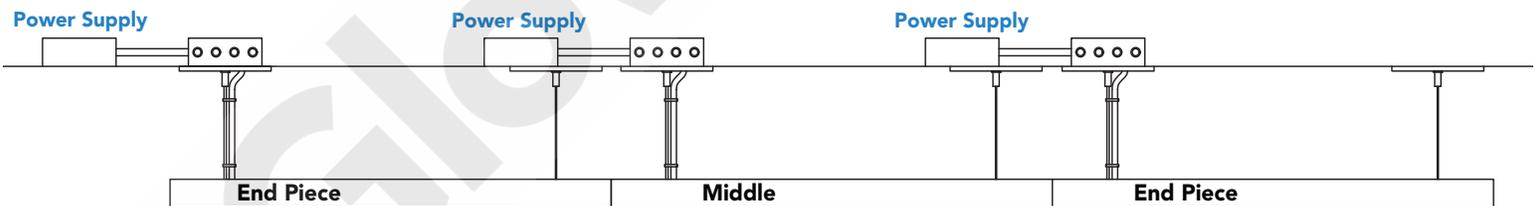
**Note:** When ordering a continuous run, specify the overall length of run needed. One of our project managers can specify the correct configuration. Continuous runs are "linkable" and consist of (2) end sections, and as many "middle" sections as needed to achieve the run.
