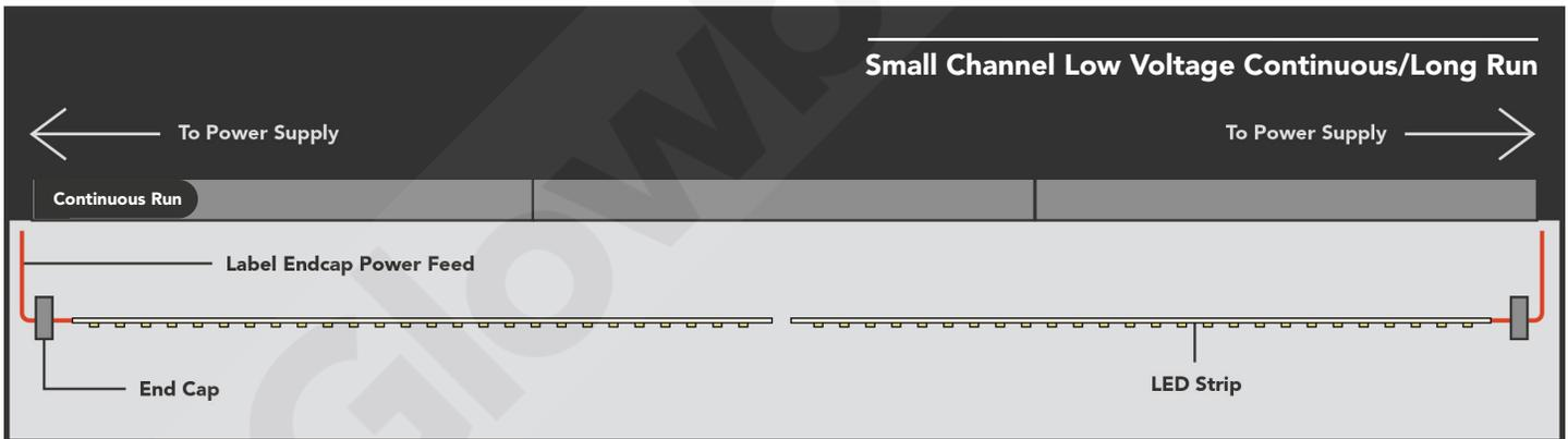
**Small Channel Low Voltage Continuous/Long Run**
