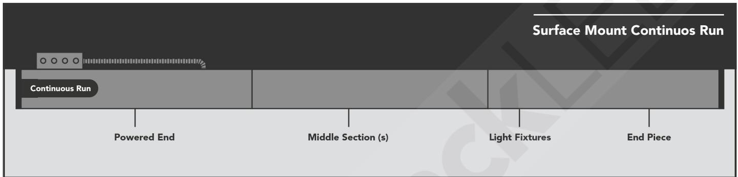
\*Fixtures do not include conduit, they have "knock-outs" to receive conduit
