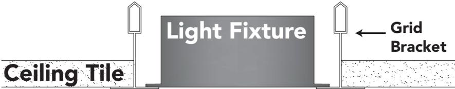
**Opening:** Refer to chart on **Page 1** for required opening size. Opening created using grid-structure.
