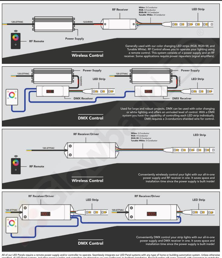
specified, all LED Panel systems, including power supplies and controllers are shipped to you pre-configured, to facilitate installation. Power-Supplies will come "rigged" with connectors to match the connectors coming off the LED panels. When ordering, simply give us some details about the level of control that you want, and our team will design a turn-key control system fit to meet your needs.
