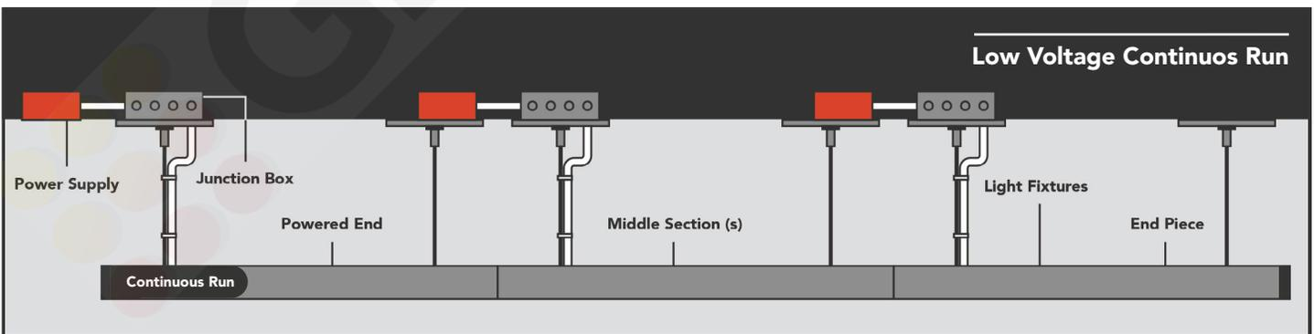
**\*Remote Power Supplies MUST be left accessible, they cannot be installed behind finished ceilings.**
